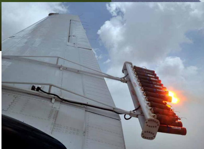
Photograph of burning hygroscopic flares during a seeding experiment in Coahuila, Mexico.
