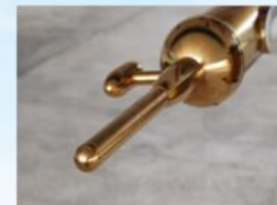
AIMMS Probe Aircraft-Integrated Meteorological Measurement System Temp., RH, Wind
