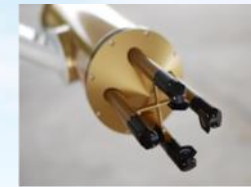
2D-S Probe A Two Dimensional, Stereo, Particle Imaging size 10 – 1280 \mu\text{m} resolution 10 \mu\text{m}/\text{pixel}
