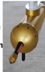
PCASP Passive Cavity Aerosol Spectrometer Probe Aerosol size 0.1-3.0 \mu\text{m}
