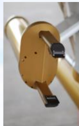
HVPS Probe A High Volume Precipitation Spectrometer Particle size 150-19,200 \mu\text{m}
