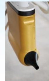
CPI Probe Cloud Particle Imager resolution 2.3 \mu\text{m}/\text{pixel}
