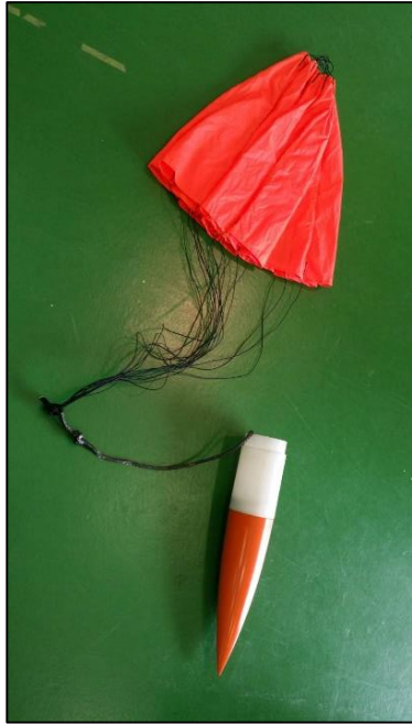
Parachute 1 for Nose Cone
